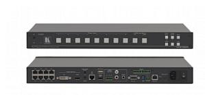
The VP-81SIDN is a high-performance digital switcher for DGKat twisted pair, DVI and HDMI signals. The unit has DVI and HDMI local inputs and eight DGKat inputs from HDMI, DVI, DisplayPort and computer graphics video step-in modules, each of which has a step-in button to select the input on the switcher
